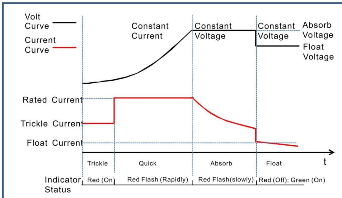
**Fig. 1 Three-stage Charging Curve**
