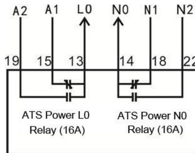
Fig.5 – Internal Wiring of ATS Power LO-NO Output
