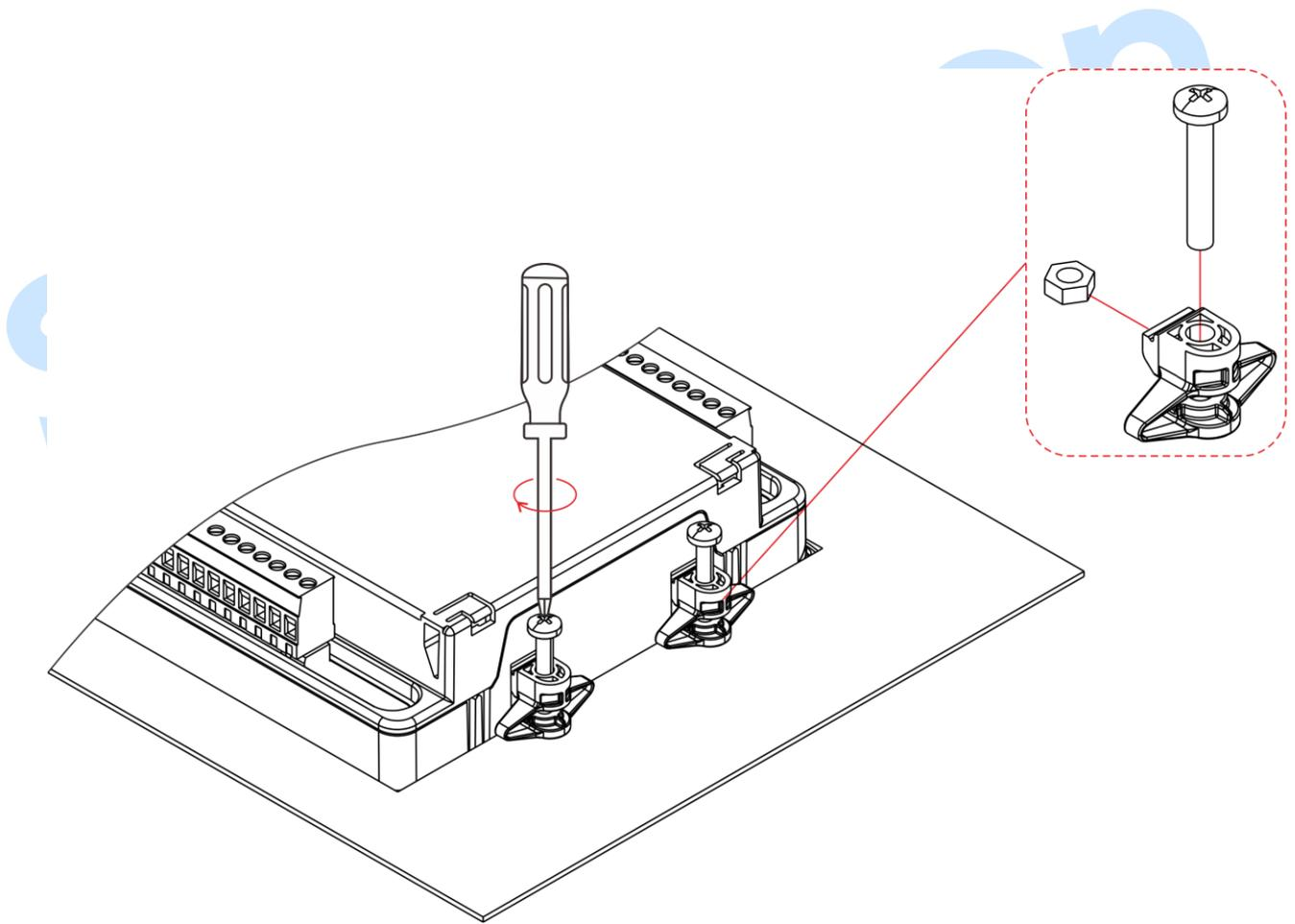
Fig.14 – Clips Installation Drawing
