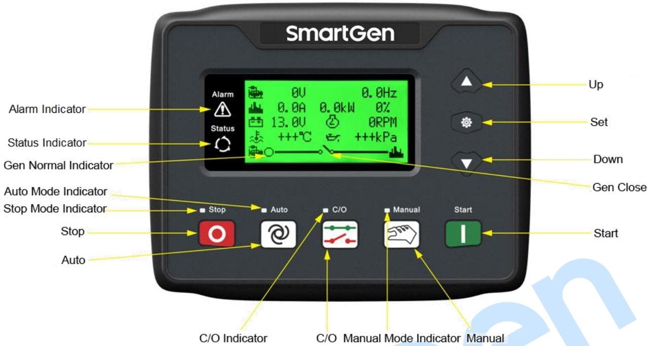
**Fig.1 HGM4100LT Front Panel Indication**
