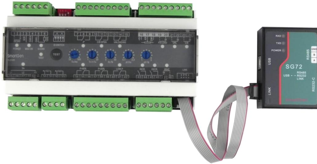
Fig. 2 - PC Programming Connection Type
