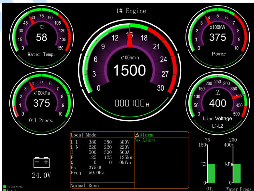
**Fig.3 Power Data Display Drawing**
